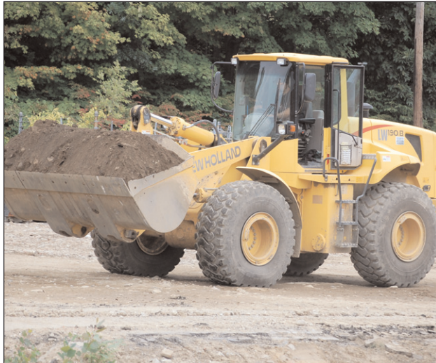
This New Holland LW190B with a 4.5-yd. (4.1 m) bucket has proven to be a workhorse.
