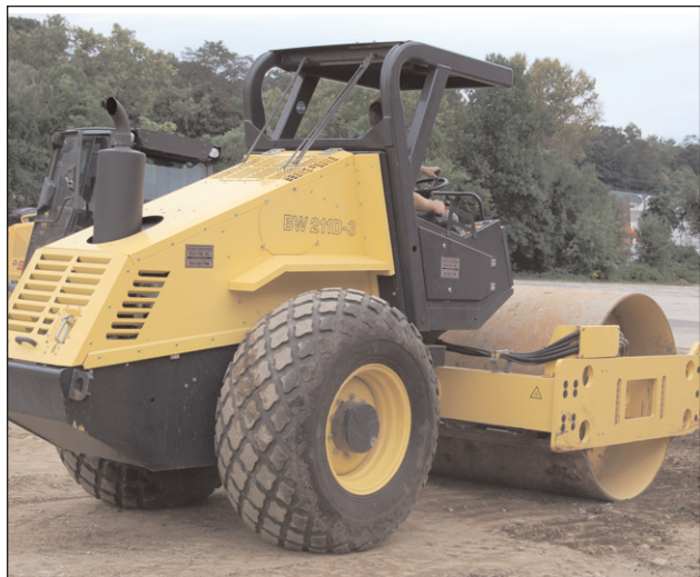
A Bomag BW211D-3 soil compactor prepares the base for a parking lot.
